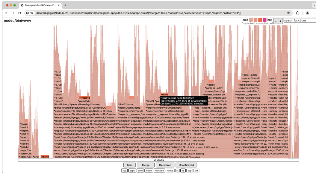
Figure 10.8 – An overview of the 0x flame graph highlighting readFileSync() as a hot frame
